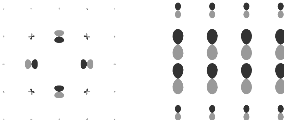
Fig. 5. Details of two 2D orientation score tensor fields, showing the degree-3 tensors as glyphs corresponding to a polar plot of |\mathbf{s}^{\odot 2} \cdot \mathbf{U}_2(\mathbf{x})| (with dark lobes corresponding to negative values). The original image for the left tensor field had a single dot in the middle, while on the right the original had ones on the top half and zeroes on the bottom. Note how the “width” of the response is inversely related to the dimensionality of the feature.
