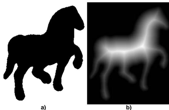
Figure 1: Object (a) and distance transform (DT) (b)
