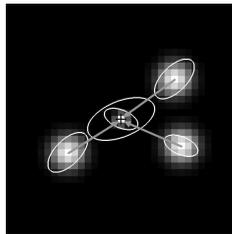
**Fig. 3.** Structure of a COSFIRE filter that is configured for the bifurcation shown in Fig. 2a. This filter is trained to detect the local geometrical arrangement of five contour parts. The ellipses illustrate the orientations and wavelengths of the selected Gabor filters, and the bright blobs are intensity maps of 2D Gaussian functions that are used to blur the responses of the corresponding Gabor filters. The blurred responses are then shifted by the corresponding vectors.
