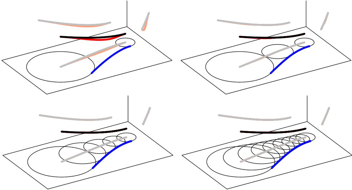
Figure 4: Conversion of an analytic curve (black) into an MPH spline in Example 1. The MPH interpolants are depicted in red, the associated PH spline in blue.
