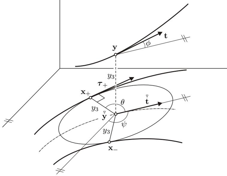
Figure 3: Spatial/planar  $G^1$  Hermite data for interpolation by MPH/PH curves (note that  $\phi$  is a hyperbolic angle).
