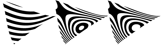
Figure 2: Reflection lines on a cubic triangle for various normal interpolation methods. Left to right: linear interpolation, quadratic interpolation for PN triangles, and the new quadratic interpolation for arbitrary PN polygons.
