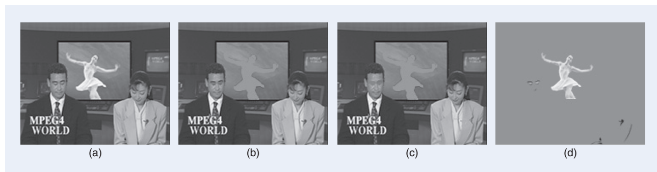
[FIG15] Example of motion connected operator preserving fixed objects: (a) original frame, (b) motion connected operator \psi , (c) dual operator: \psi^*\psi(f) , and (d) residue: f - \psi^*(\psi(f)) .
