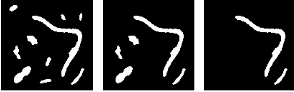
Fig. 3. Binary attribute filters applied to an image of bacteria: (left) original; (middle) area opening using area threshold \lambda = 150 ; (right) elongation thinning using attribute I/A^2 > 0.5 .
