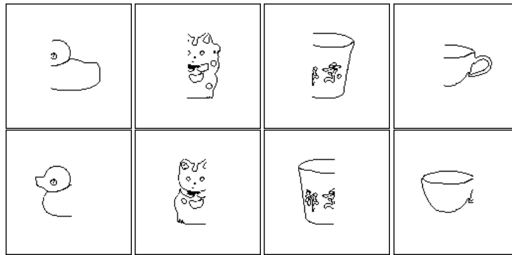
Fig. 5. Ocluded contour representations of objects. The images are obtained by removing 30% of the contour from left (row 1) and right (row 2).
