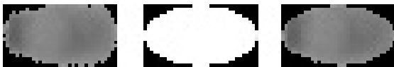
Fig 4. The rotated image is re-scaled to 19x35 pixels (left). We apply an elliptic mask of 19x35 pixels (center) in order to define the 2D grey level function f(x,y) (right).
