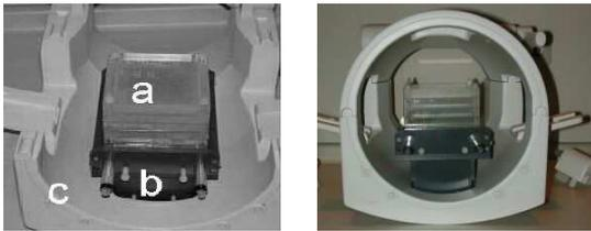
Fig. 14. Oblique view (left) and horizontal view (right) of the phantom (a) together with the motion device (b) inside the MRI head coil (c). Two pistons and two adjustment nuts are also visible.
