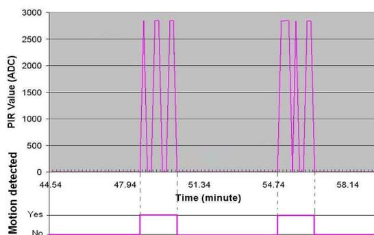
Figure 3: PIR Sensor Data
