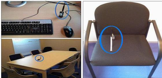
(b) Acoustic Sensors' Placement (c) Pressure Sensor Placement
