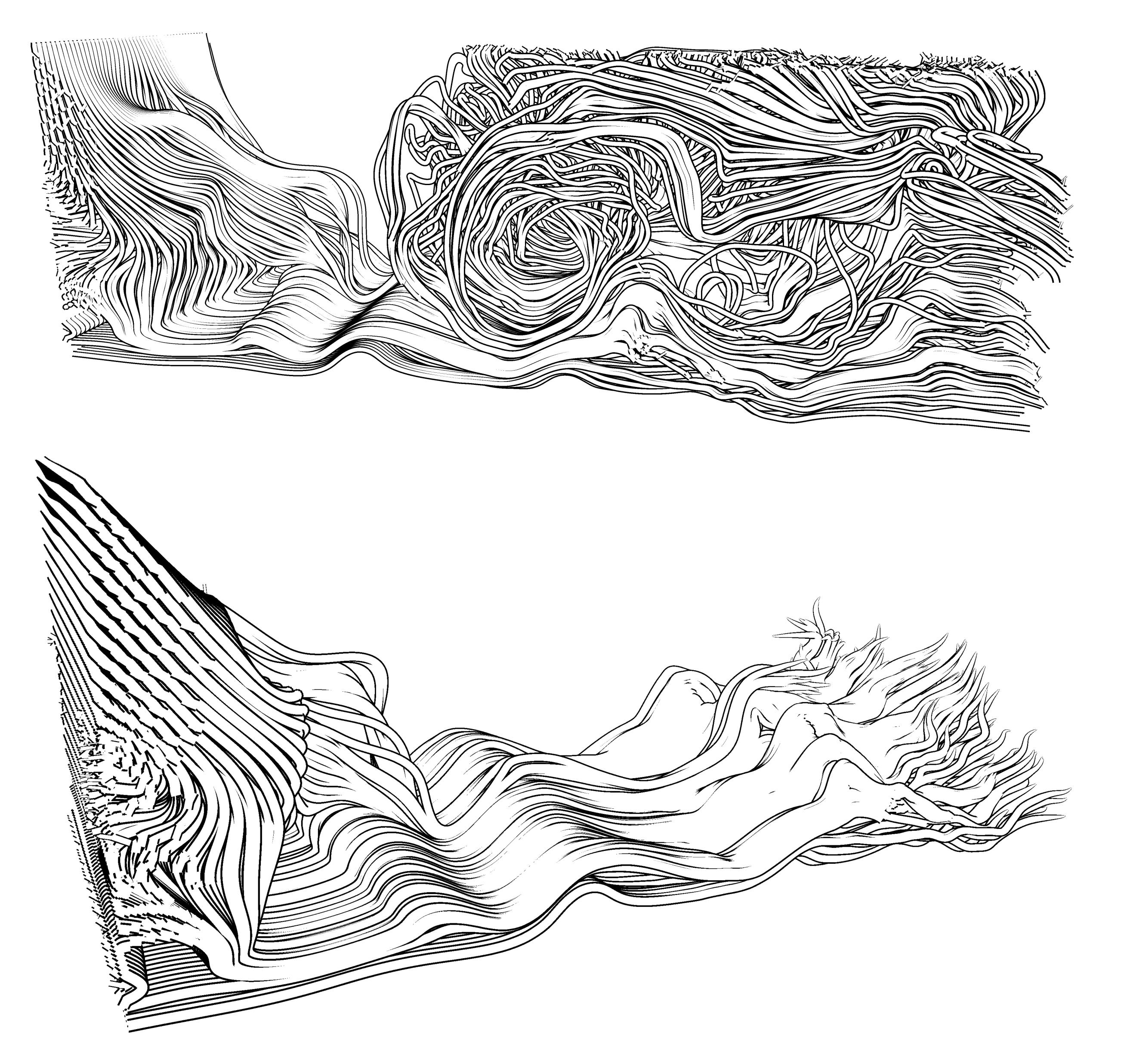
The depth-dependent halo technique merges individual streamlines into structure-emphasizing bundles. The parallel nature of streamlines and their relative depth is clearly conveyed.
