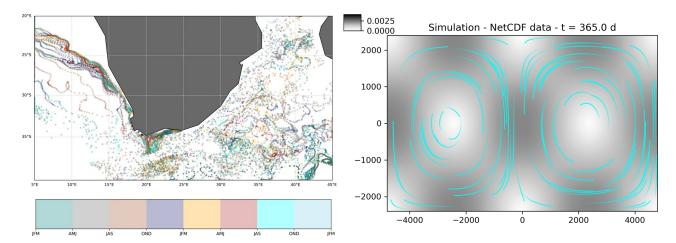
In *computational fluid dynamics (CFD)* and oceanography, the tracing of particles in hydrodynamic fluid velocity fields is used to study the particles transport and their behaviour in Newtonian fluids. Such fluid dynamics study is called *Lagrangian simulation*, as the particles trajectory form through Lagrangian integration of their positions over time. The field of directional, hydrodynamic velocity tensors is the underpinning *Eulerian model*.
