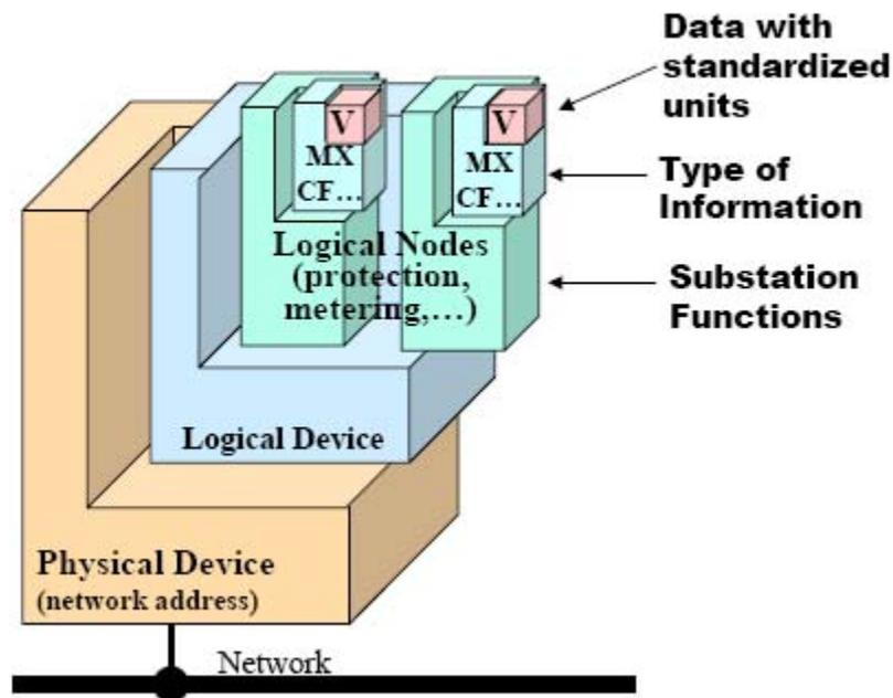
Figure 13: IED containing the logical nodes [18]
