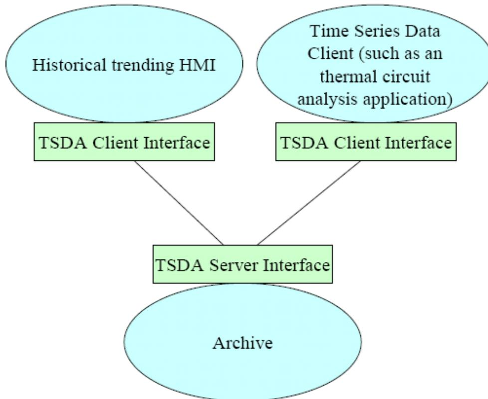
**Figure 12: TSDA client and server exchanging an archive of data [15]**
