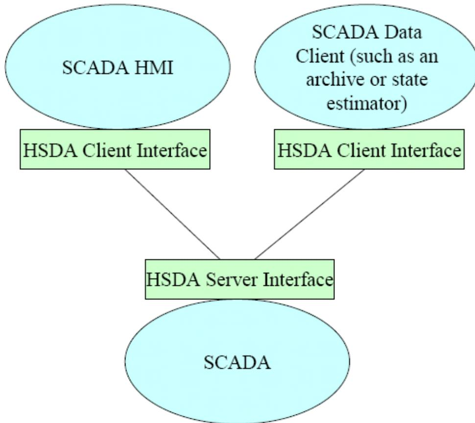
Figure 11: HSDA and SCADA system [15]
