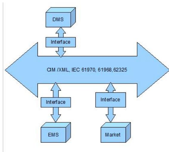
Figure 15: Communication bus which will accommodate more standards
