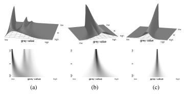
Fig. 4. (a) Histogram of a noisy MR image, (b) histogram of the difference between a noisy MR image and the noise-free MR image, and (c) histogram of the difference of two noisy MR images, for various  $\sigma$ . Top: surface plots, bottom: grey value maps.
