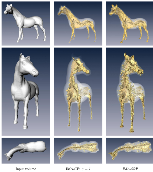
Fig. 5. Volume renderings of binary horse data ( 128 \times 280 \times 232 voxels) and its skeletons (side, front and top views). First column: input data. Second column: IMA-CP skeleton with \gamma = 7 . Third column: IMA-SRP skeleton. In the skeleton renderings, the input volume is rendered partially transparent.
