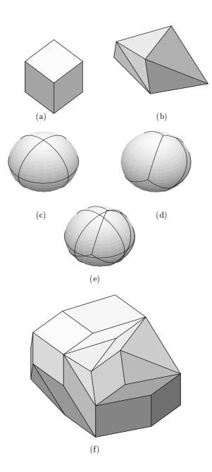
**Fig. 1.** Two polyhedra A and B (a) (b), their slope diagrams SDA and SDB (c), (d), the overlay of these slope diagrams SDC (e), and the Minkowski sum C of the polyhedra A and B, (f). It may take some time to see the relation between (b) and (d). It can be seen that the (f) consists of the faces of (a) and (b), and additional parallelepiped faces (See also figure 3b). MSR methods calculate (f) directly from (a) and (b). MSD methods use the slope diagrams in (c), (d) and (e) to calculate (f).
