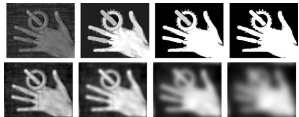
Fig. 5. Alternating top-hat and bottom-hat scale spaces filtering example. First row: f_0, f_{12}, f_{20}, f_{25} ; second row: Gaussian diffusion filtering at time t = 4.5, 12.5, 50.0 and 112.5 .
