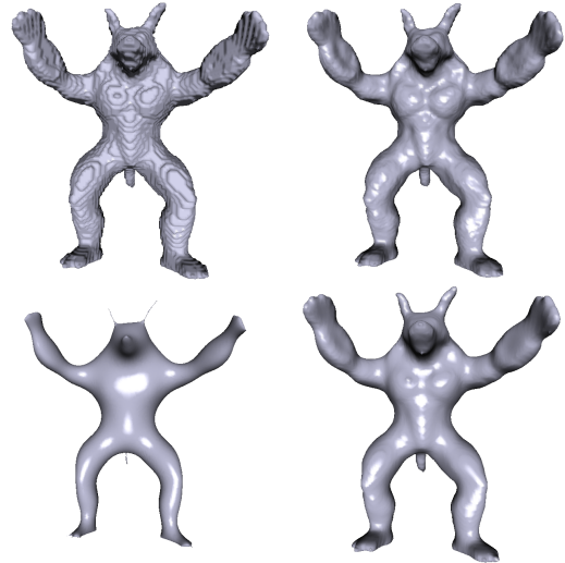
Figure 6: Mesh smoothing comparison. Left-to-right, top-to-bottom: original mesh, method of Jones et al. [JDD03], curvature flow [MDSB03, DMSB99], our method.
