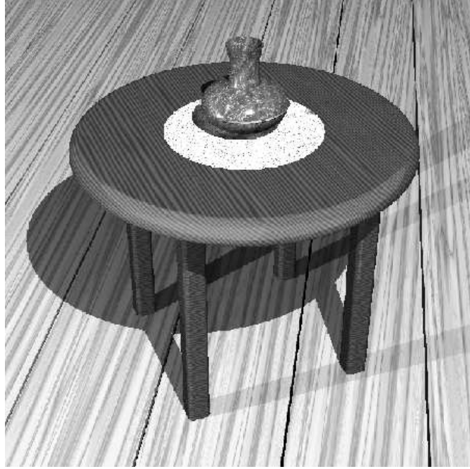
Figure 6: Legs and blade of the table are modelled by Minkowski sums.
